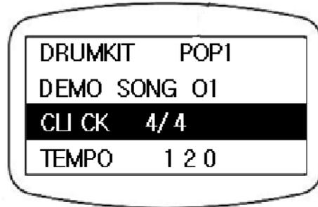
When the CLICK option is highlighted, users can press the SETUP button for further settings.
