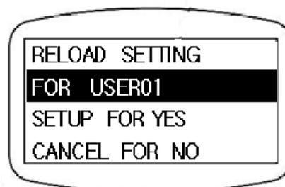
User can press LEFT/RIGHT button to select the drum kit to be reloaded. Press SETUP after selected drum kit to restore setting or press CANCEL button to quit.
