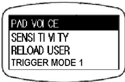
When the PAD VOICE option is highlighted, press the SETUP button again to enter the submenu to change the settings of a drum pad voice as illustrated below
